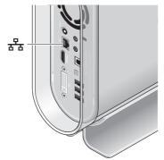
Use only an Ethernet cable (RJ - 45 connector). Do not plug a telephone cable (RJ-11 connector) into the network connector.
