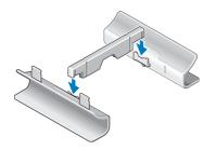
Align the securing tabs on the stand with the slots on the computer and lower the computer onto the stand until the securing tabs are inserted into the slots.
