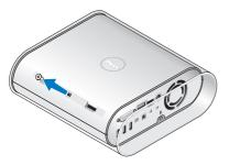
2. Place the computer vertically and pull the sleeve gently towards the back of your computer, then gently slide the new sleeve onto the computer.
